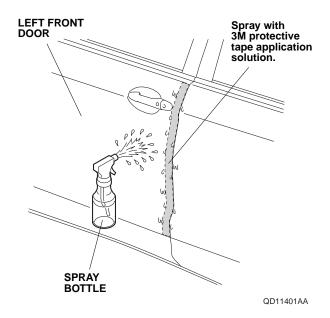
Open the left front door. Peel back about 50 mm (2.0 in.) of adhesive backing from the left front door edge film. Align the V-notch on the left front door edge film with the character line on the left front door.
